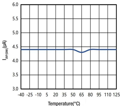
Fig. 1  $I_{UVP(SNK)}$  vs Temperature
