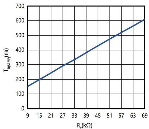
Fig. 12. T<sub>D(SAMP)</sub> vs R<sub>T</sub>
