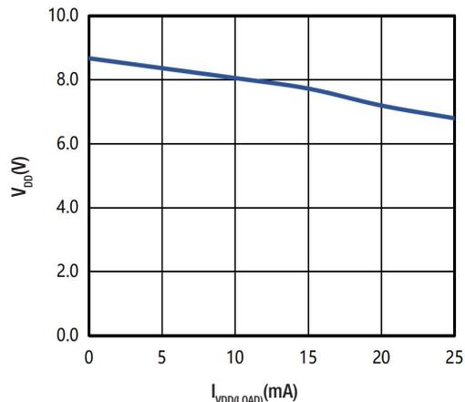
Fig. 8. V<sub>DD</sub> vs I<sub>VDD(LOAD)</sub>
