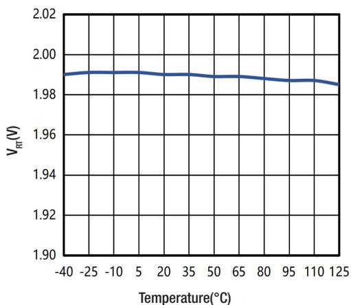
Fig. 3  $V_{RT}$  vs Temperature
