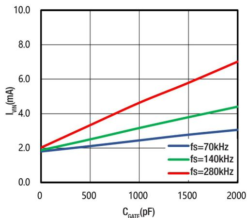
Fig. 10. I<sub>VIN</sub> vs C<sub>GATE</sub>
