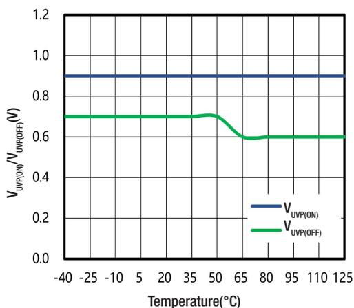
Fig. 5  $V_{UVP(ON)}/V_{UVP(OFF)}$  vs Temperature
