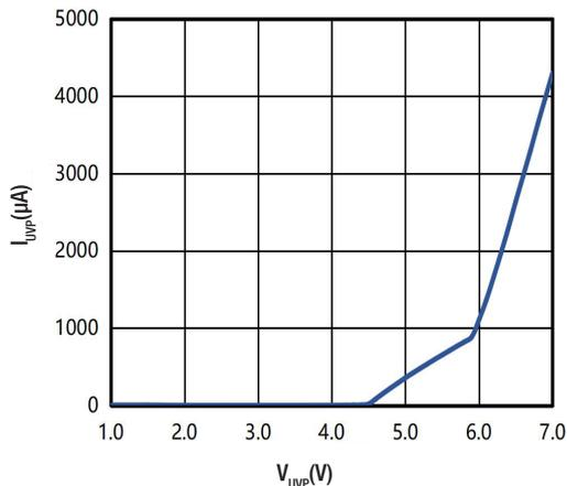
Fig. 7. I<sub>UVP</sub> vs V<sub>UVP</sub>
