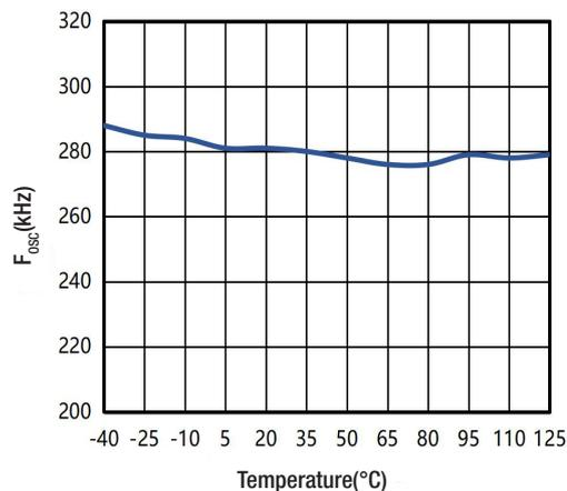
Fig. 2  $F_{osc}$  vs Temperature @  $R_T=22k\Omega$
