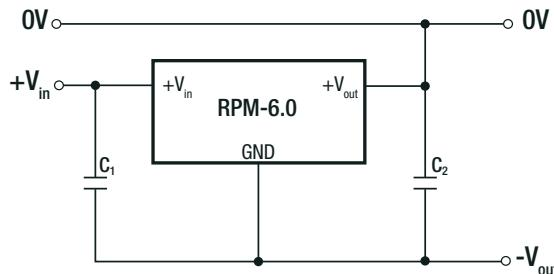
**C<sub>1</sub>** and **C<sub>2</sub>** may be added to reduced ripple and should be fitted close to the converter pins.
