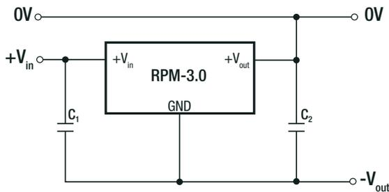
$C_1$  and  $C_2$  may be added to reduced ripple and should be fitted close to the converter pins.
