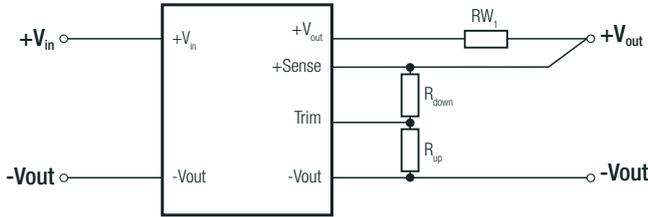
The output voltage can be adjusted via the trim and sense functions.
