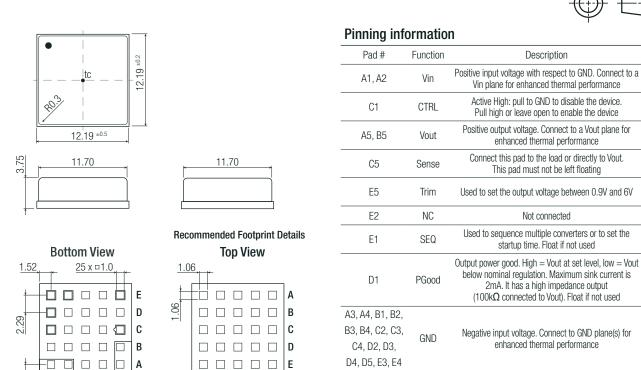
tc = case temperature measuring point Pad tolerance= ±0.05mm Case tolerance=  $\pm 0.25$ mm
