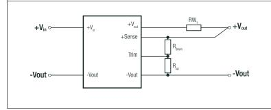
The output voltage can be adjusted via the trim and sense functions. The maximum output voltage from Trim and Sense function combined is 5.5VDC. Derating may be required when using Trim and/or sense functions.
