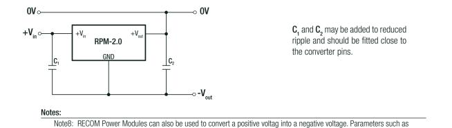
maximum Vin, efficiency and maximum operating temperature are reduced. Please contact RECOM for further details.
