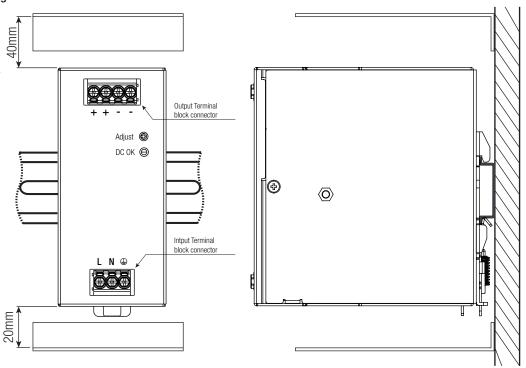
Note8: To guarantee sufficient convection cooling, keep a distance of 40mm above and 20mm below the device. For vertical mounting the device should be installed with the input terminal on the bottom.
