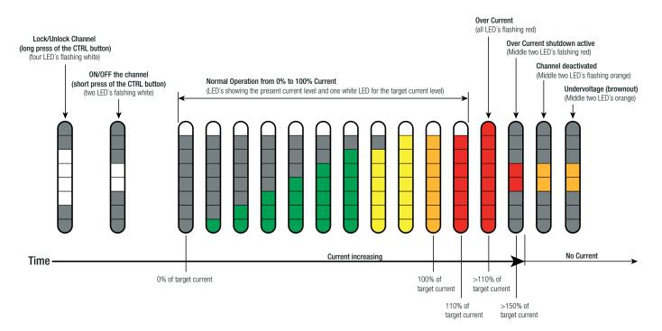
Actual current: Colored LEDs indicate the actual current of 0-110% in relation to the set maximum current. In the picture above the target current is set to it's maximum.
